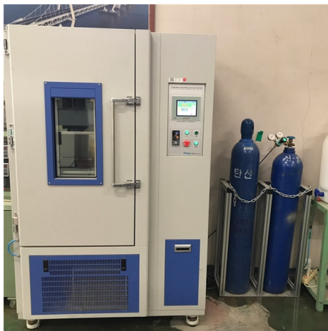
Fig. 6 Accelerated carbonation testing equipment
