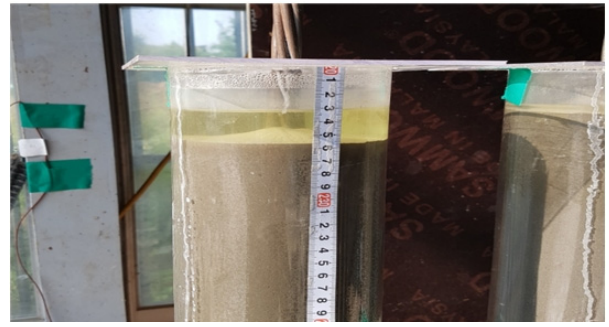
Fig. 6 Photo for bleeding of grout A (W/C 0.45)
